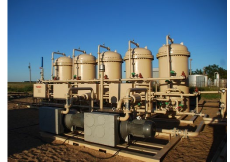
Modular units used to treat the raw gas stream to remove nitrogen, CO2 and concentrate helium
