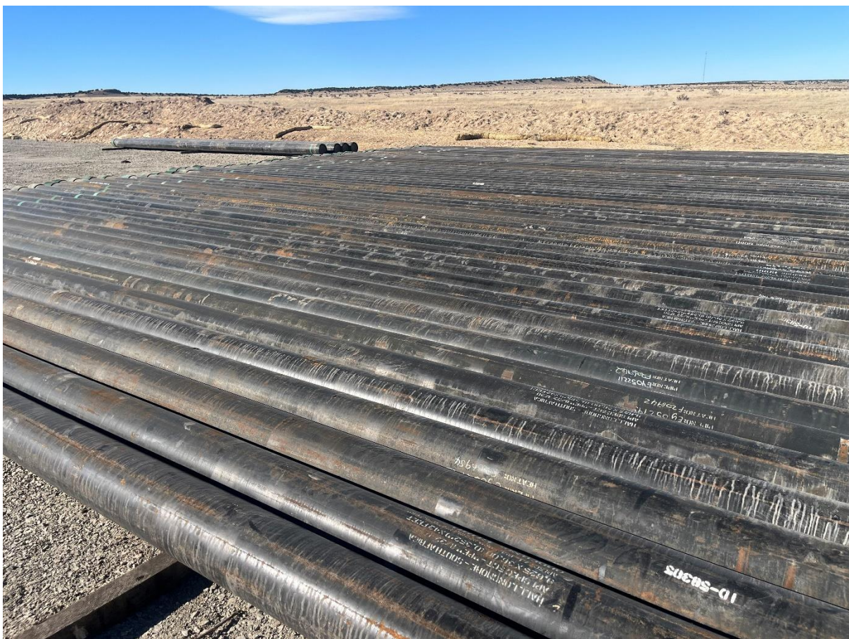
Casing and conductor for multiple wells on location
