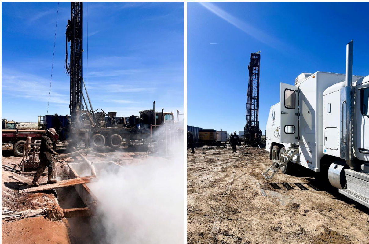
Air drilling the Lyons Sandstone (left) and open-hole logging of the Lyons at TD (right)
